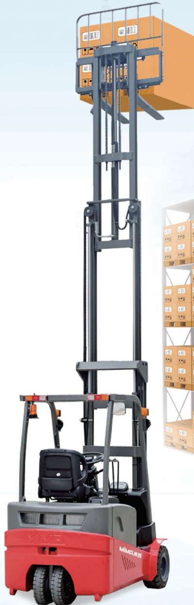
TKC series dual front-wheel drive counterbalanced forklift
